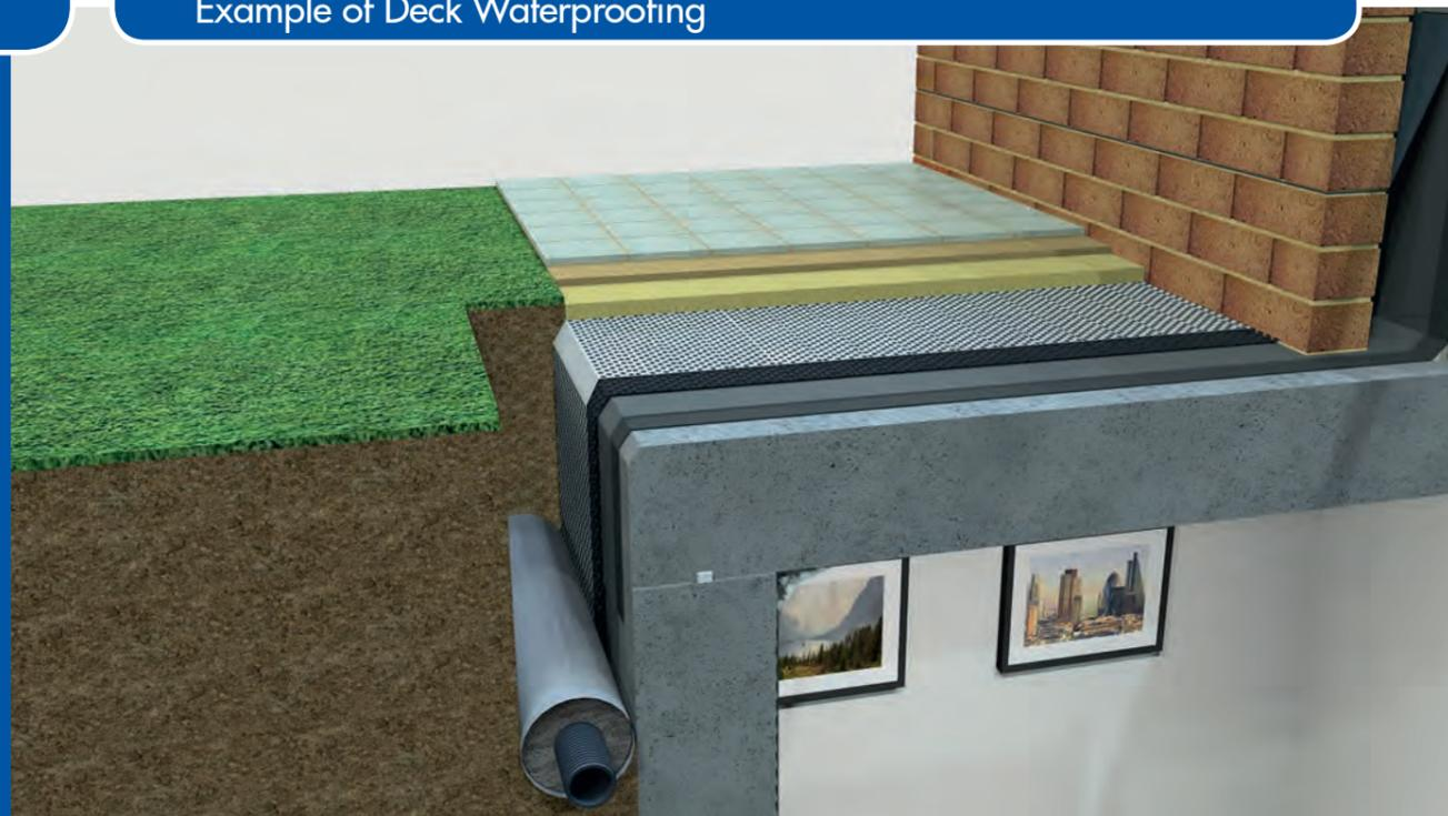
The Newton DeckFlex System providing multi-coat liquid-applied waterproofing to an inverted warm roof
